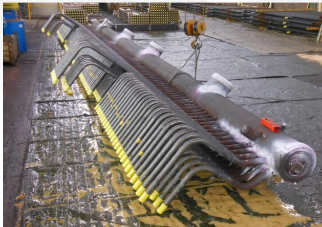
ECO inlet header within fabrication
