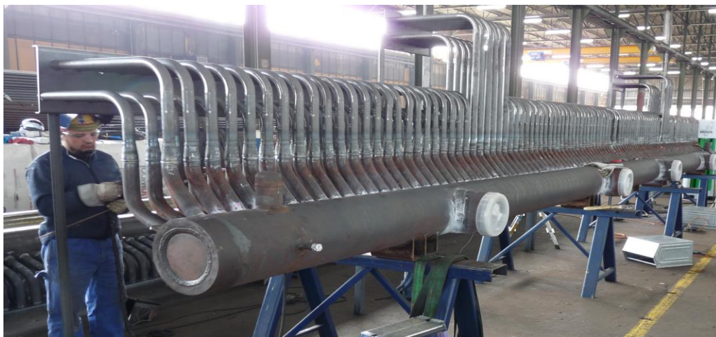
ECO inlet header within fabrication
